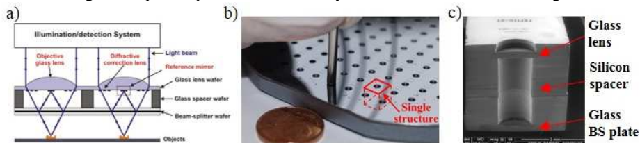
Fig 1. Micromachined Mirau micro-interferometer: a) schematic view [1], b) wafer-level fabrication result (Si-Glass-Si-Glass structure) [2], c) cross-section of individual Mirau structure
